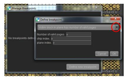
Choose a breakpoint type from the scroll down menu. The relevant parameters for this type will appear. Edit the parameters you are interested in and press OK.
